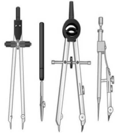
Figure 3-19 – Bow instruments: bow pen/pencil; bow divider, bow drop pen drawing instrument set
